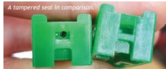
Figure 20: Example of a tampered seal in comparison to an untampered seal
