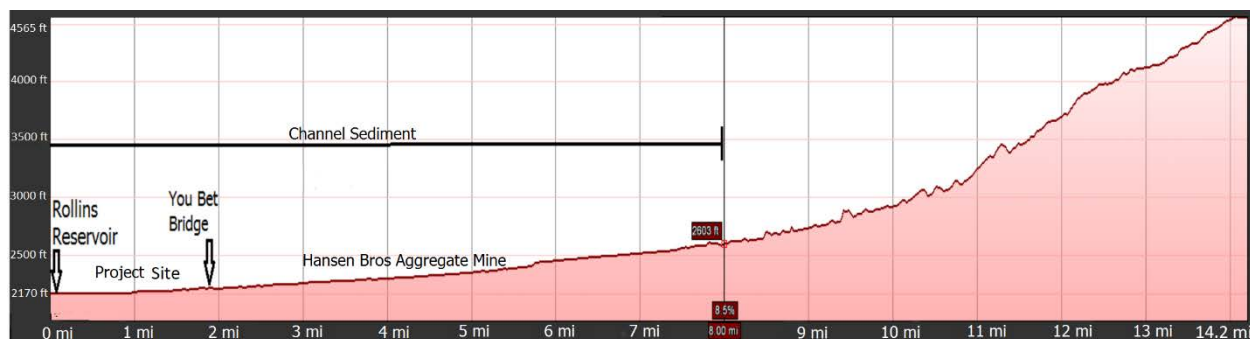
Figure 3.8-1 Greenhorn Creek Channel Elevation/Gradient
