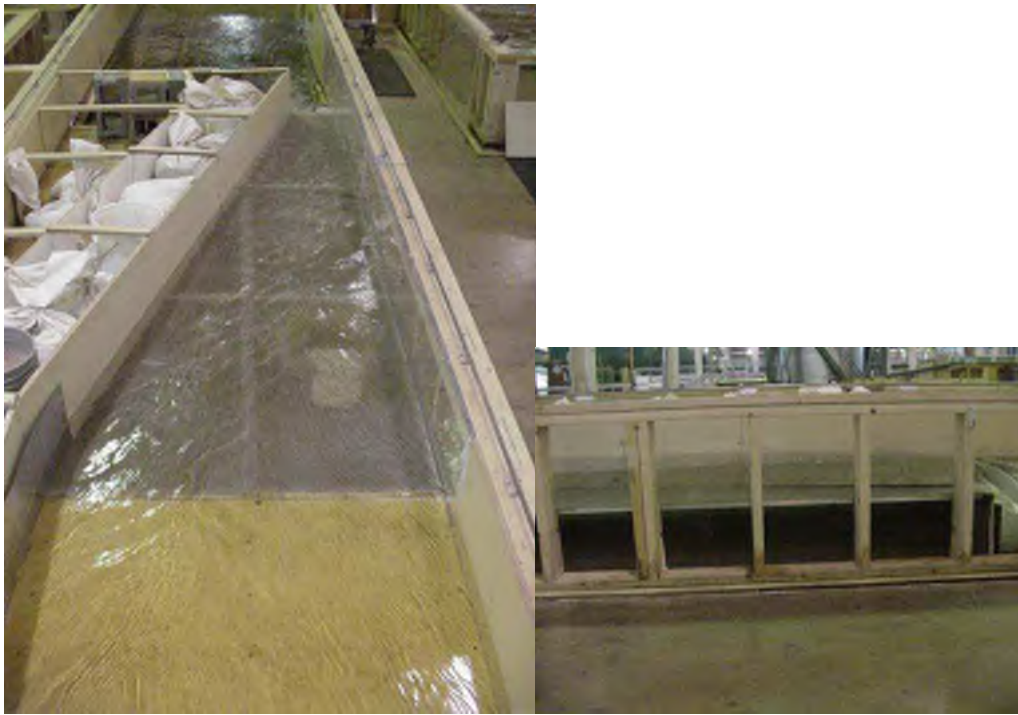
Figure 27.—Test 20. Critical flow at the downstream end of the screen with Q_c = 4.07 \text{ ft}^3/\text{s} and Q_d/Q_c = 67 percent. Flow depth of 0.5 ft. The sweeping velocity is increasing across the screen and particularly as the flow enters the bypass opening. The approach velocity in the last foot of the screen is positive indicating that flow is coming up through the screen.
