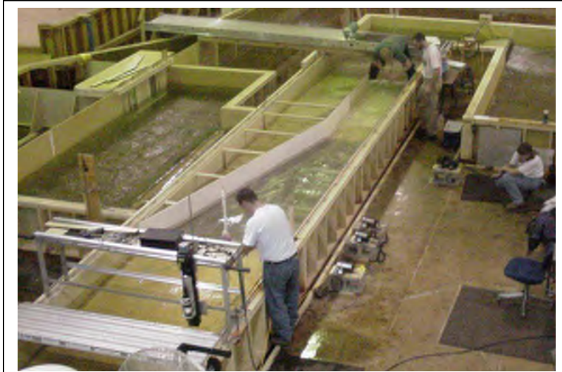
Figure 35.—Bull trout testing with the 15-degree converging wall over the screen.
