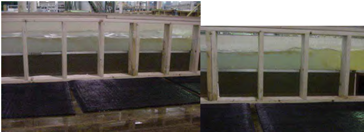
Figure 7.—Top and side views of test 3 with supercritical flow at the upstream end of the screen transitioning to subcritical with a jump over the downstream end of the screen. Q_d/Q_c=0.55 and V_a=0.115 ft/s. The upstream V_s/V_a = 44:1 , and the downstream V_s/V_a = 20:1 , with the channel discharge, depth, and screen width used to compute the sweeping velocity. Compare to test 1 and test 2 with same approach velocity, depth, and V_s/V_a=5 and 10 to 1.
