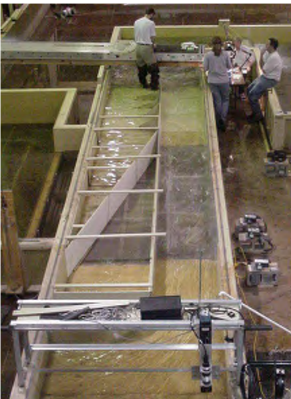
Figure 36.—Control test setup for bull trout testing with clear plastic over the screen and 2 ft/s sweeping velocity.
