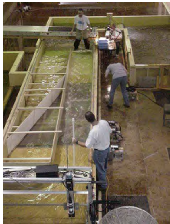
Figure 37.—Control test setup for bull trout testing with clear plastic over the screen and 4 ft/s sweeping velocity.
